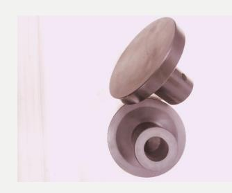
This fixture has the purpose of determining the mechanical properties of unreinforced and reinforced rigid plastics, including high modulus composites, when loaded in compression at relatively low uniform rates of straining or loading.
