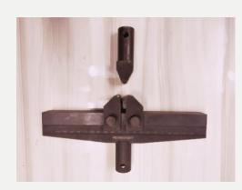
This fixture meets the requirements of ASTM D2344 for testing the short-beam strength of fiber-reinforced polymer-matrix composite materials and laminates. The fixture has a 6 mm diameter loading nose and 3 mm diameter support rollers, as specified in the standard for testing flat beam samples. The support span is adjustable from 4 to 150 mm with the ability to test specimens up to 30 mm wide.
